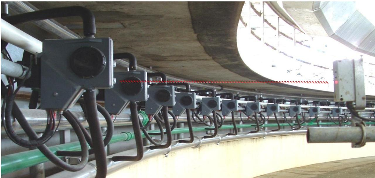
1. The RTO (remote take off) can determine if the Automilker is still milking at the point when the infra-red beam aligns with the Automilker, just before the exit on the platform and turns the Automilker off.
